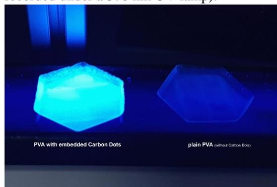
As could be noted, the PVA-Carbon Dots composite present a strong photo-luminescence located in the blue region of the visible spectrum compared with the plain PVA sample. The long term UV ageing tests were started using an UV-C source but, unable to be finished due to the premature stopping (end of April 2022) of the research project.
