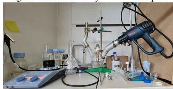
tube able to withstand high temperatures and rapid cooling of the reaction mass through flooding with water, a surrounding glass mantle
