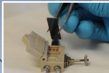
the microcell setting-up into the fluidic cell
