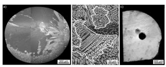
Figure 1: IQ-maps of microstructure cross sections through beads produced via levitation melting: a) polycrystalline b) dendritic and c) single crystalline.
