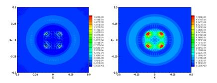
Figure: Non-well-balanced methods: The contours of the pressure and velocity perturbation of a two dimensional hydrostatic solution with  $100 \times 100$  cells at t=0.2. Left: pressure p. Right: velocity  $\sqrt{u^2+v^2}$ . Notice the different contour range.
