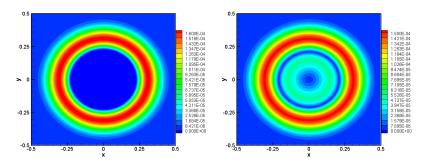
Figure: Well-balanced methods: The contours of the pressure and velocity perturbation of a two dimensional hydrostatic solution with  $100 \times 100$  cells at t=0.2. Left: pressure p. Right: velocity  $\sqrt{u^2+v^2}$ .
