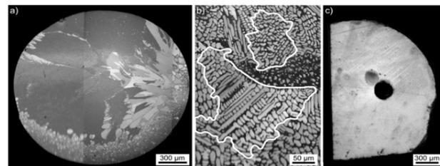
Figure 1: IQ-maps of microstructure cross sections through beads produced via levitation melting: a) polycrystalline b) dendritic and c) single crystalline.
