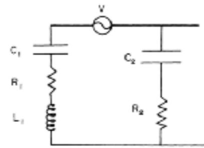
FIG. 4. The equivalent circuit of the detector and transducer.
