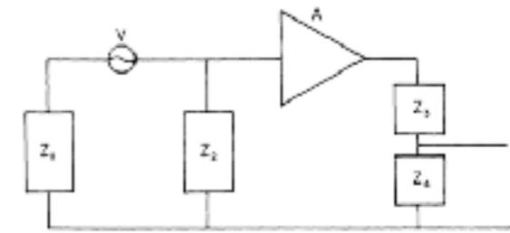
FIG. 5. The equivalent circuit for discussing the signal/noise ratio.
