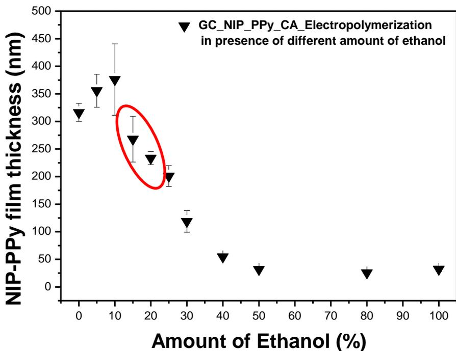
The evaluation of NIP-PPy film thickness with amount of ethanol present in solution
