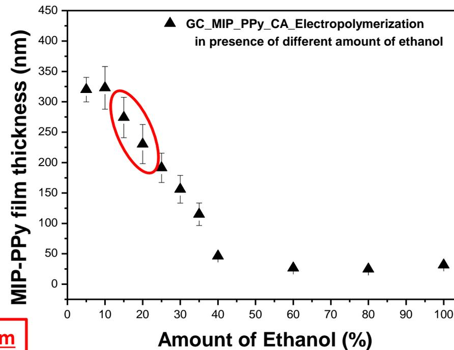
The evaluation of MIP-PPy film thickness with amount of ethanol present in solution
