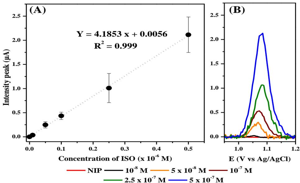
The calibration plot is found to be linear between 0 and  $5 \times 10^{-7} \text{ M}$  and obeys to the following relation:
