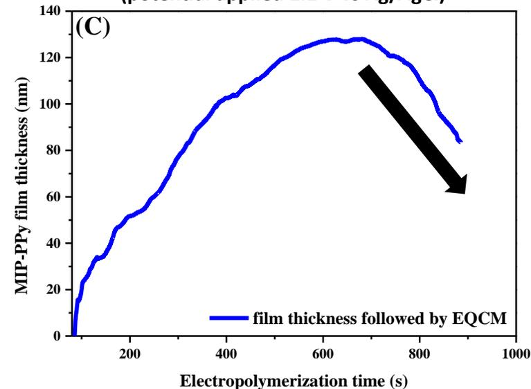
EQCM study of anodic polypyrrole film growth on gold quartz electrodes by chronoamperometry 1000 sec (potential applied 1.1 V vs Ag/AgCl)
