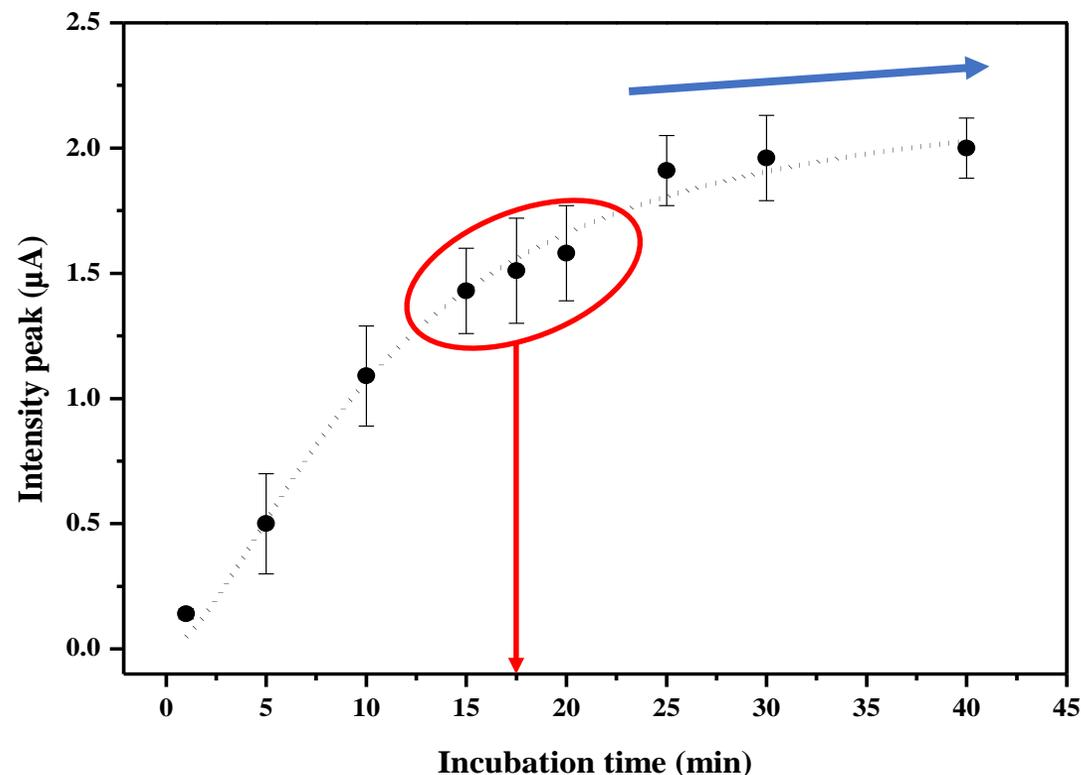
The adsorption time for the GC-MIP-PPy electrode was optimized to be 15 to 20 mins
