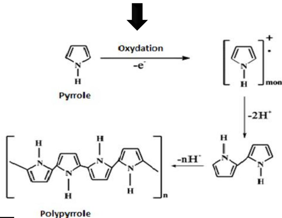
*a radical coupling mechanism*
