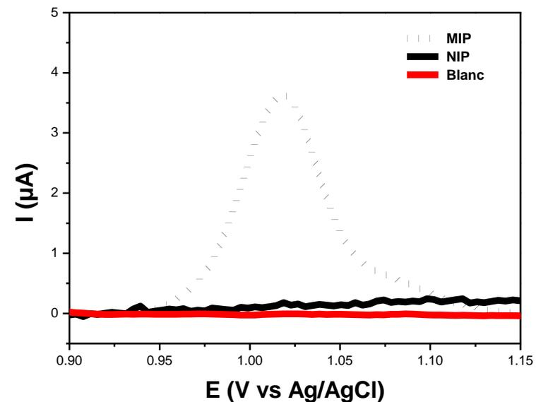
SWV detection of isoproturon
