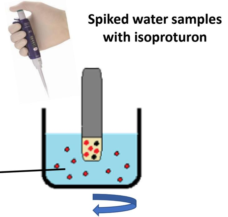
Rebinding of GC-MIP-PPy sensors in different isoproturon concentrations prepared in milli Q water ( $18.2 M\Omega.cm$  at  $25^\circ C$ )
