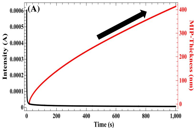
The polypyrrole film growing by electropolymerization duration times 25 sec up to 1000 sec (potential applied 1.1 V vs Ag/AgCl)
